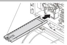
**5** Close the maintenance cover, and press the ENTER key. The warning will be reset.
