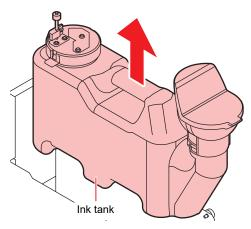
(3) Press the protrusion on the lid of the ink tank and reace a new ink tank.
