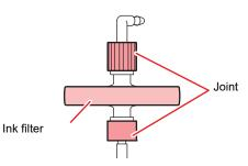
(3) Remove the joint attached to the side of ink fillter.
