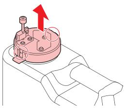
(4) Set a new ink tank, and mount the ink filter.Tighten the joints on the top and bottom of the ink filter.
