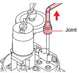
(4) Set a new ink tank, and mount the ink filter.Tighten the joints on the top of the ink filter.
